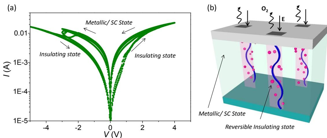
Figure 1- (a) Bipolar resistive switching measured in a YBCO layer with silver contacts. (b) Schematic representation of the creation of reversible pinning potentials in a YBCO film based on the local modulation of the oxygen content by means of an electric field.
