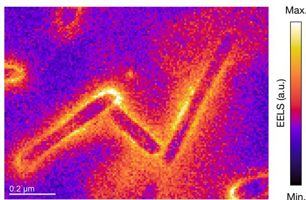
**Figure 1.** Experimental study of low-loss EELS acquired in MoS<sub>2</sub> nanotubes. Intensity map of the EELS signals integrated for a energy-loss window between 1-2 eV.
